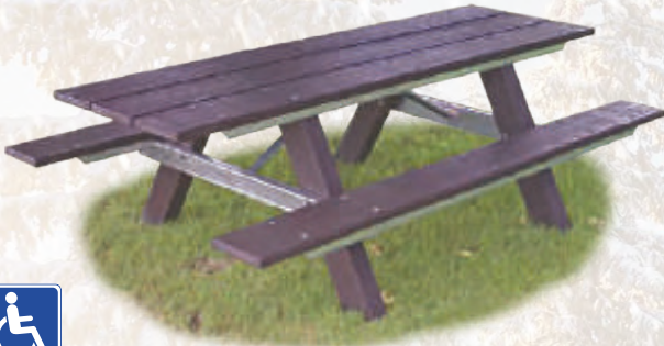
Model WAT-8 A-Frame Table 8 ft. long and wheelchair accessible at both ends. The table structure uses Recycled Plastic leg posts and top/seat planks and incorporates steel braces for support. This table was tested to hold over 500 lbs. per sq. ft. load without failure. (see Page 37)
