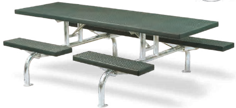
Model T603/G-8DN surface mount table, one long seat, two short seats (total 3 seats), hot dip galvanized frame, 8 ft., thermo-plastic coated expanded steel in green color.
